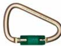
Steel Carabiner 5005I Length: 4.88" (124mm), Opening: .94" (24mm), Breaking Strength: 9,218 lbs. (41kN)
