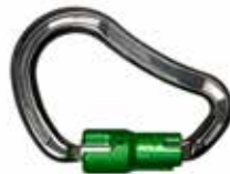
Aluminum Carabiner 5555S3 Length: 4 7/8" (123.83mm), Opening: 3/4" (19.05mm), Breaking Strength: 6,744 lbs. (30kN)
