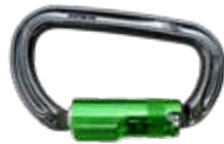
Aluminum Carabiner 5555S4 Gate Opening: .63" (16mm) Length: 5 5/8" (142.87mm) Breaking Strength: 6,744 lbs. (30kN)
