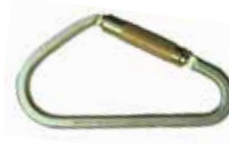
Steel Carabiner 5005L1 Length: 7 5/8" (193.68mm), Opening: 2 1/8" (53.98mm), Breaking Strength: 8,992 lbs. (40kN)
