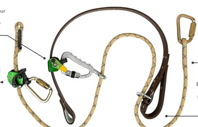
New wear-resistant Tough Rope is constructed with an energy absorbing nylon core, red braided polyester inner core cover (red wear indicator) and an abrasion and heat resistant Technora outer jacket that eliminates the need for a wear guard.
