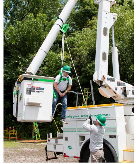
4:1 pulley system allows for easy lifting of injured worker. Photos used for demonstration purposes only. Always wear your PPE.
