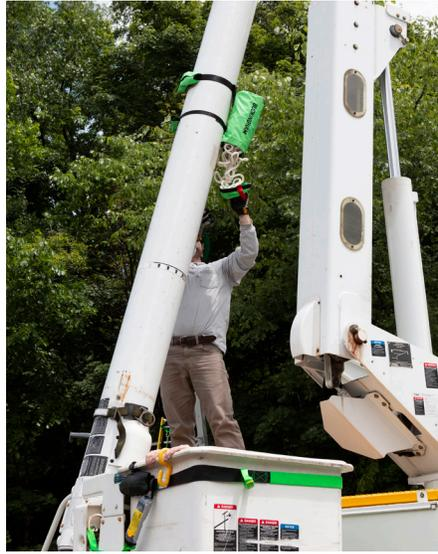
In case of rescue situation, simply tear away the cap with the red webbing and components will drop out easily and freely.
