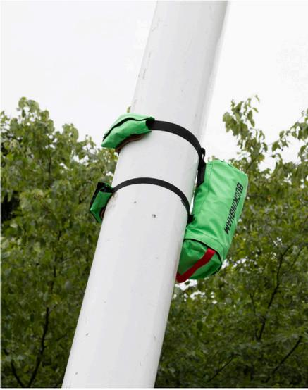
Newly designed setup allows for hurt man rescue system to be permanently attached to boom without risking damage to components because of weather. Gum rubber allows for secure placement on the boom.
