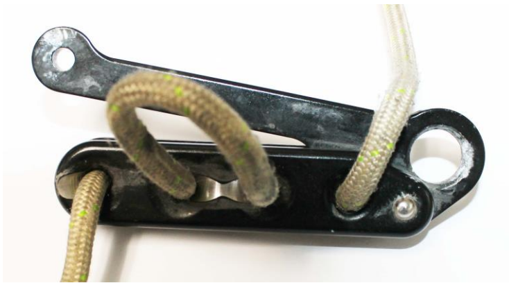
CORRODED DESCENDER WITH EXCESSIVE WEAR GROOVES / MARKS FROM DESCENT LINE FRICTION
