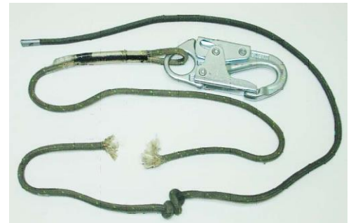
CUT / BROKEN ROPE
