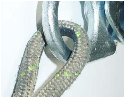
EXCESSIVE WEAR INSIDE OF EYE
