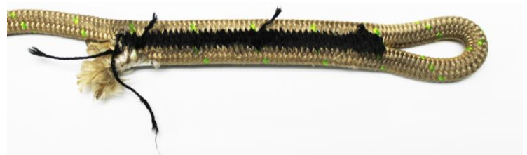
BROKEN / PULLED / CUT STITCHING
