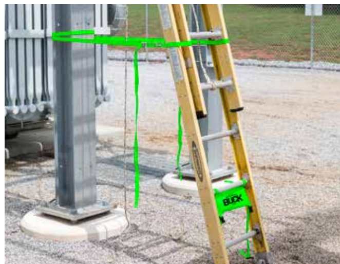
Ladder Lock (model 355B) used to secure ladder to steel prior to working.
