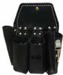
Double Back Holster 42266-BL Remains rigid & prevents tight fitting tools from bending and buckling the back of pouch when removing tools. Features 5 pockets and a 2-way knife snap. Measures: 10.75" L x 8" W
