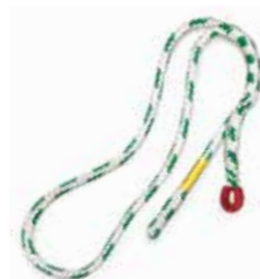
OX TAIL™ 39078TAG1-4 4' x 5/8" adjustable sling. 39078TAG1-7 7' x 5/8" adjustable sling. WLL: Straight 3200 lbf. Choker 2560 lbf. Basket 6400 lbf.
