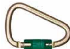
Steel Carabiner 5005 Length: 4.88" (124mm) Opening: .94" (24mm) Breaking Strength: 9,217 lbs. (41kN)
