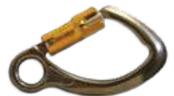
Aluminum Carabiner w/Eye 5005SAE Length: 5.25" (133mm) Opening: .71" (18mm) Breaking Strength: 5,620 lbs. (25.5kN)
