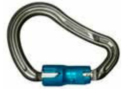
Aluminum Carabiner 5555S2 Length: 4.80" (122mm) Opening: .78" (20mm) Breaking Strength: 6,730 lbs. (30kN)
