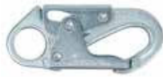
Steel Locking Snap Hook 1706 Gate Opening: 1 5 / 16 " Eye Opening: 1" (25mm) Length: 6" (152mm) Rated to 5,000 lbf (22kN)
