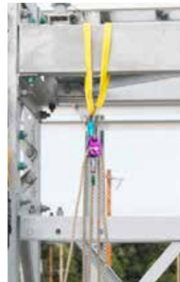
2. Raise victim with Rescue Blocks and progress capture.
