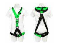
The New BuckArticulator™ Dielectric "Y" Style Harness was developed for the worker that deals with electrical hazards; making this a great option for substation and other linemen work. Dielectric hardware eliminates the potential of static electricity being transferred through steel hardware if working around an energized conductor in wet or damp conditions. Also, Dielectric hardware has a better resistance to corrosion in extreme conditions (hot or salty air environments).
