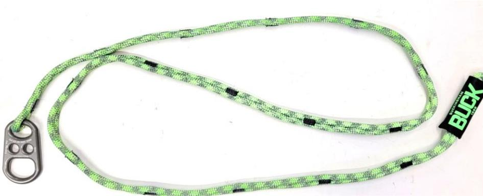
The PN 65-10 SuperBase Anchor (10 ft. long) was developed with ArborMaster. This Basal / Base anchor is used for anchoring an Arborist's climbing line at the base of the tree. It can be set up in multiple configurations, see below. Setting up the anchor at the base of the tree also allows the climber to rig for rescue, allowing for a ground-based rescue in the event of an emergency.
