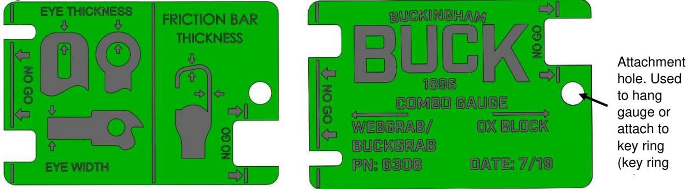
The Buckingham Mfg. PN 6308 OxBlock – WebGrab Combo Inspection Gauge (Fig. 1) is designed to check the friction bar thickness on all OxBlocks and the eye thickness and width of the WebGrab and BuckGrab supplied on our SuperSqueeze, EZSqueeze, BuckAdjuster and SuperStrap products. (Fig. 2 – 5)
