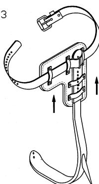
Slide the climber pad along the shank of the climber onto the sleeve, aligning the sleeve loop with the loops on the horizontal leg of the pad. Insert climber strap in the direction shown, through the pad loops and the climber sleeve loop. See Fig. 3 ('right' climber shown). Note: Foot strap must be attached to the leg iron stirrup in the same direction as shown for the calf strap.
