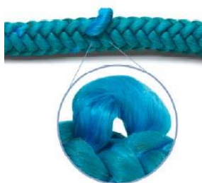
Rope with a Pulled Strand
