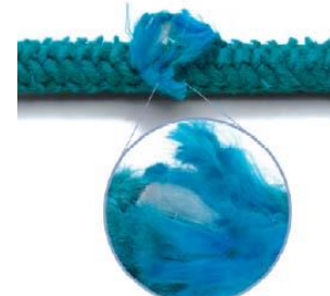
Rope with Broken or Cut Strands
