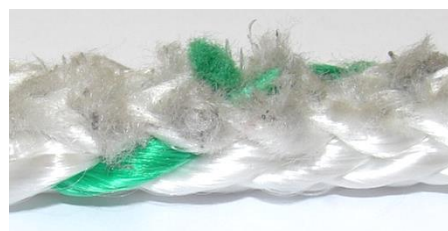
Rope with Excessive Abrasion / Wear
