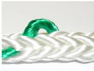
Rope with a Pulled Strand
