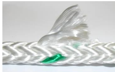
Rope with Broken or Cut Strands
