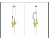
The ZIGZAG PLUS mechanical Prusik is used on either doubled ropes or a single rope, thanks to the CHICANE accessory, which offers more friction on the descent, and the KNEE ASCENT assemblies, which facilitate the ascent.
