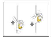
In normal use, the ASAP mobile fall arrester moves freely along the rope to accompany the user in all his movements.
