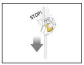
In case of a sudden movement (fall, slide, uncontrolled descent...), the fall arrester locks on the rope and stops the user.
