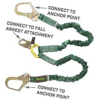
**Warning:** Dual lanyards must be used in a manner in which the energy absorber pack is not bypassed as this will render it ineffective as an energy absorbing lanyard and in the event of a fall, result in impact forces exceeding OSHA requirements.
