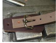
5) Place a copper burr over rivet. 6) Seat the burr onto the rivet shaft. (Use tool/method appropriate to seat burr)
