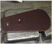
4) Fold buckle strap over rivet and into next hole.
