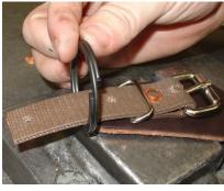
13) Insert a tall rivet through the chafe & 2 buckle strap holes. Attach a burr, seat, & peen same as shown in steps 5 through 9.
