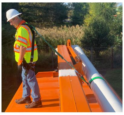
Great for use when working on a chipper box of a bucket truck to remove snow. Simply choke the sling to the boom and hook in with your bucket harness and lanyard. Sling slides easily along the boom and you have access to the full chipper box and headache rack.
