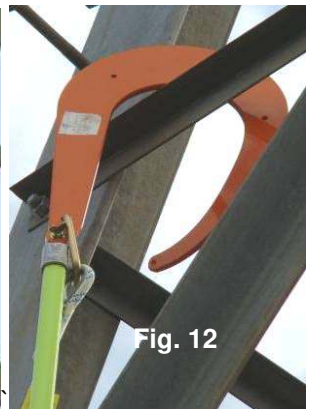
b. Insert rope into channel of Fall Arrester
