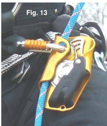
c. Attach carabiner to Fall Arrester
