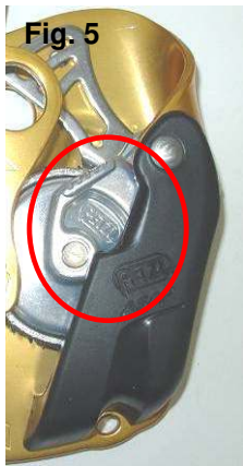
a. Depress silver button on side of locking wheel
