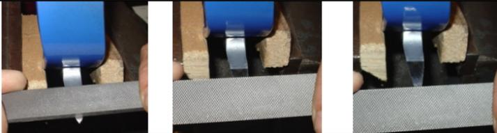
Keep file flat, push away from the gaff heel toward the tip and roll the file "over-and-down" at the tip to maintain proper tip radius. This radius is the **KEY** to proper pole penetration. It forces the gaff deeper into the pole with less effort. Gauge your work frequently. Touch up with the hone PN 6501 and climb with assurance.
