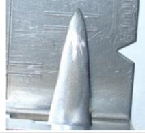
If the gaff tip, when inserted through each of the Thickness Check Steps, fails to fit between the inscribed lines on the gauge, the gaff is either:
